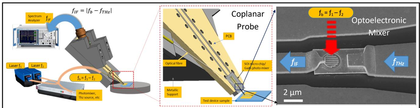
Figure 1: Principle of optoelectronic mixing on coplanar probe for broadband characterization of dynamic electrical properties of THz components on wafer. The signal's frequency,  $f_{THz}$ , is converted to a low frequency,  $f_{IF}$ , for analysis by a standard measuring instrument, directly on the measuring probe by the optoelectronic mixer, which is pumped by an optical frequency beat  $f_b = f_{THz} \pm f_{IF}$ .
