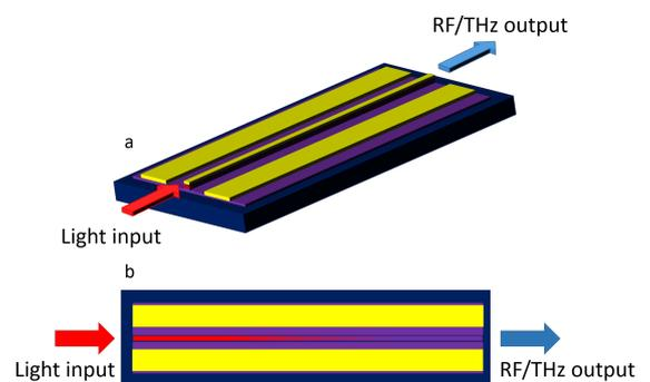
Figure 1 : (a) Schematic representation of a TW-photomixer. (b) Top view of a TW-photomixer showing the absorption of the optical input along the device resulting in the RF/THz generation.
